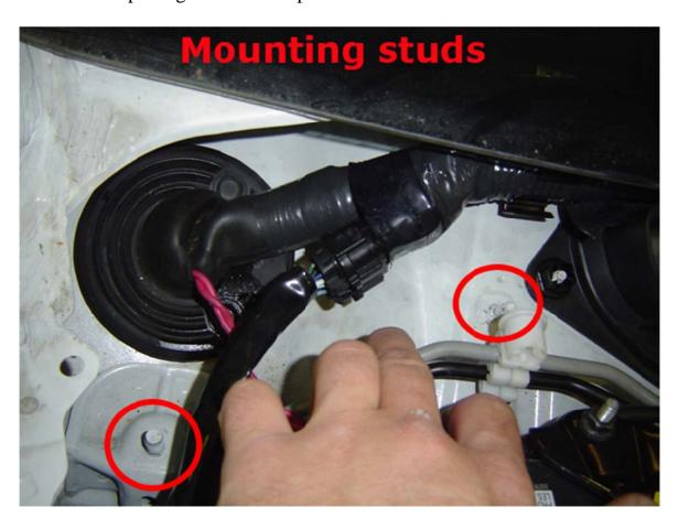
5. Put the shield in place and bolt it down using the supplied M8 nut and the plastic nut. The nylon nut goes underneath the line mount and then the line mount can go back on top of it.
