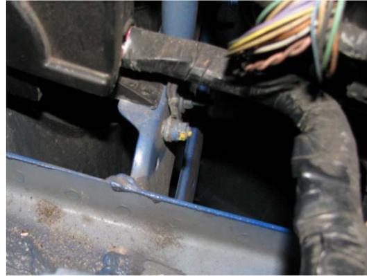
You can now feed the silicone hose through into the inner wing area and sit it into place on the channel that originally housed the standard airbox feed. The larger diameter end needs to be pushed through with the small diameter end pointing roughly towards the engine intake hose.
