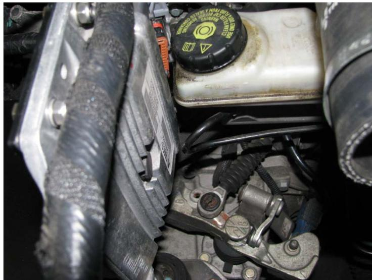
You can now plug the ECU back into wiring harness ensuring that the grey latches are fully down and secure.
