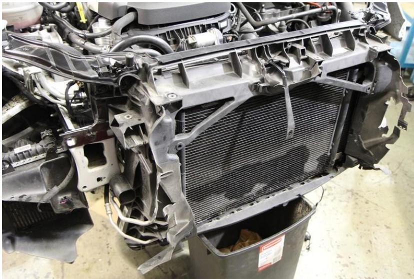
Step 8: Remove the factory clips holding the FMIC in place. WD40 is your friend here.
