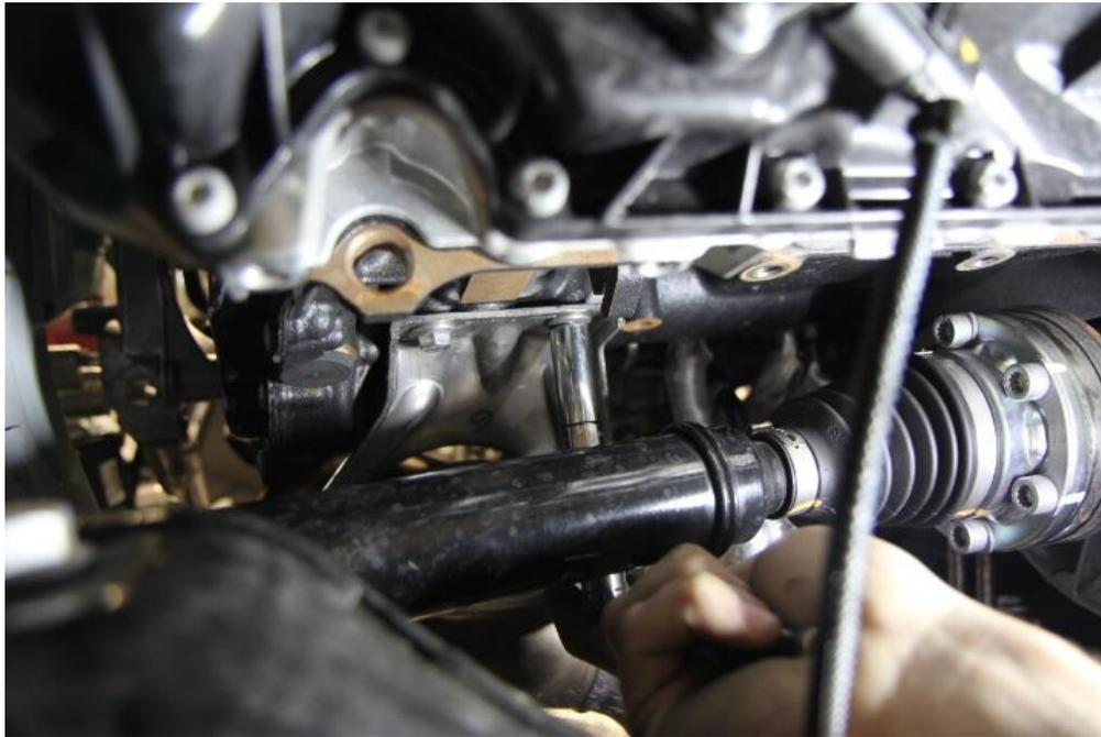
**Step 8:** Use the exhaust hanger removal tool to separate the hanger from the oem downpipe. Reinstall the hanger on the CTS High Flow Downpipe.
