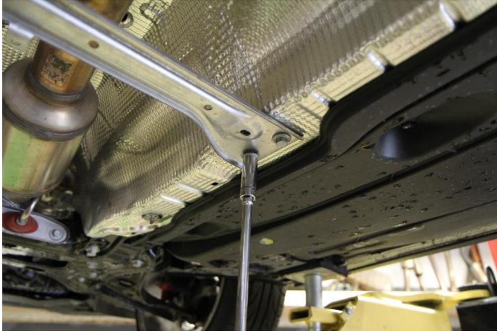
**Step 4:** Use the 16mm wrench to remove the 2 bottom bolts of the heatshield.
