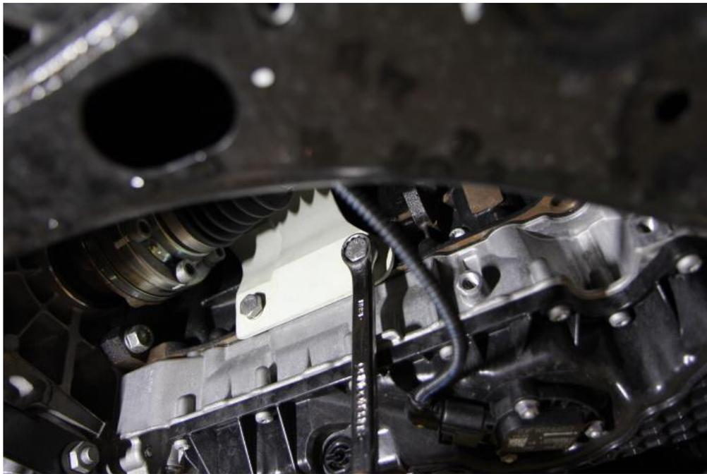
**Step 5:** Use the 13mm socket to undo the 2 bolts holding the oem exhaust clamp. Slide the exhaust clamp towards the rear of the car and allow the downpipe to hang down.
