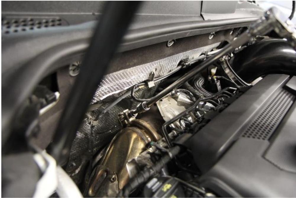
**Step 2:** Lift the vehicle on jackstands or hoist. Using a 22mm wrench or O2 sensor removal tool, remove the O2 sensor from the downpipe.
