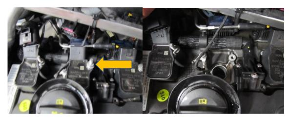
11. With the coil pack removed you can access all three T20 torx screws that hold the oil breather to the rocker cover. Undo these screws and remove that end of the breather hose.
