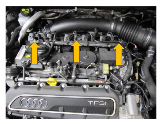
9. Unplug the three coil packs in the picture and the two sensors
