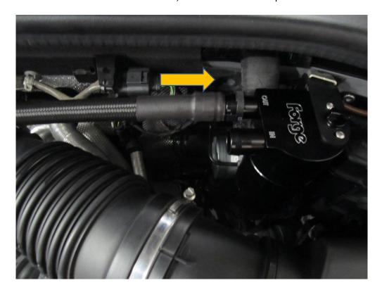
15. Using the remaining shorter hose from the catch can kit push fit the rectangular oil breather adaptor remember to push till it clicks. Now attach it to the rocker cover using the three T20 torxs screws removed earlier.
