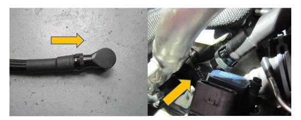
14. With the other end of this breather hose, connect it to the OUT-put of the catch can.
