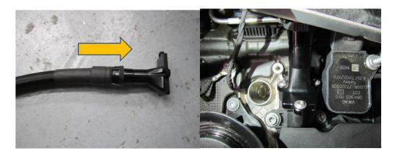
16. Re fit the coil pack, the three coil pack plugs and the two sensor plugs. The re fit the tree 10mm nuts that hold the wiring loom rail.
