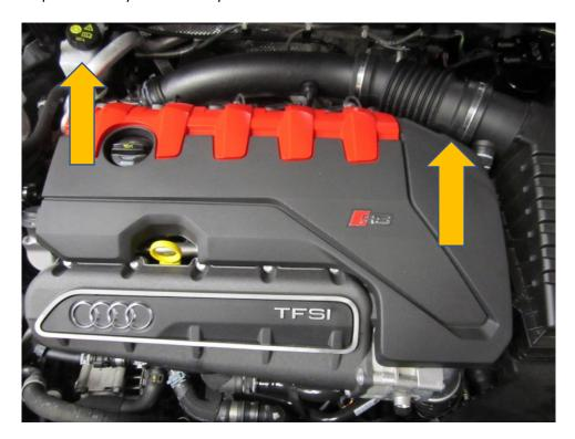
8. Undo the three 10mm nuts that hold the wiring loom rail to the rocker cover. These screws are located where the arrows are in the picture.
