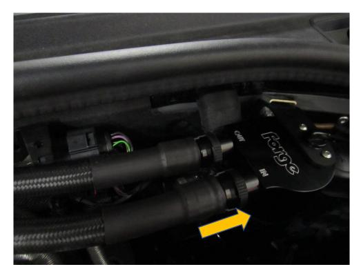
18. Attach the hose clamp to the two hoses where they naturally touch. Tighten the clamp using a 5mm Allen key.
