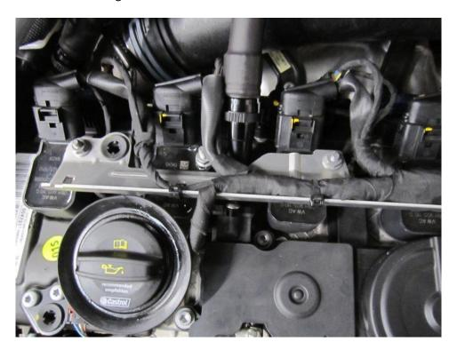
17. Connect the 2nd breather hose you have fitted to the IN-put of the catch can. Like before, it's a push fit.
