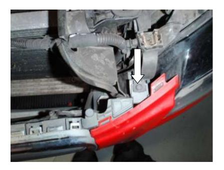
11. Using a 10mm socket undo the bolt inside both wings. These are the final fixings holding the bumper to the vehicle.
