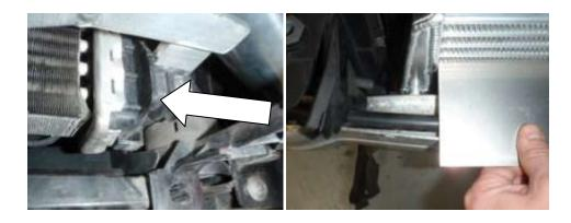
22. Remove the crash bar from the car. Continue the marked position down the front and rear face of the crash bar.
