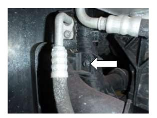
19. Un-clip the intercooler and twist top forward to release the intercooler.
