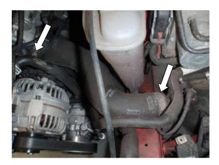
34. Undo the standard hose running to the hard pipe and resonator under the left hand wing.
