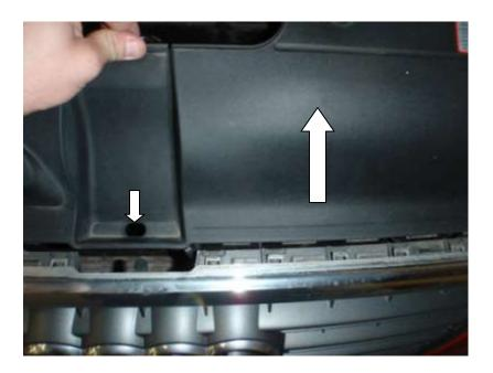
6. Disconnect the two sensors located inside the front bumper.
