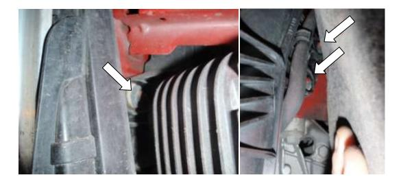
38. Undo 10mm nut located behind chassis rail.
