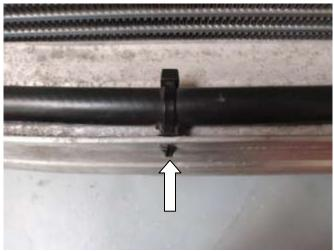
15. Using a 13mm socket or spanner undo the 4x bolts at both ends of the crash bar and remove it from the vehicle.
