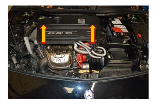
2. Using an E11 socket remove the three fasteners that hold the OE heat shield in position.
