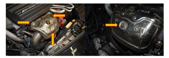
2. Disconnect the wiring loom to the lambda sensor by depressing the plastic tab on the plastic clip while pulling in opposite directions.
