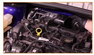
18. Remove the bolt and stud that secure the intake pipe to the valve cover.(1x 8mm bolt, 1x 12mm stud)
