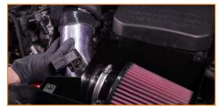
32. Secure the coupler to the intake pipe and elbow with the two worm gear clamps you installed earlier.
