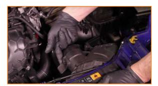
15. Remove the bolt that secures the front section of the intake pipe to the valve cover. (1x 8mm bolt)
