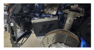
11. Using a 13mm and a 16mm socket, remove the six (6) bolts securing the auxiliary radiator bracket and remove the bracket from the vehicle. One of the lower bolts can be loosely reinstalled to keep the lower bumper reinforcement in place.
