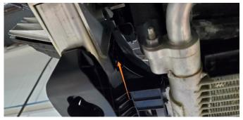
13. Using a 13mm socket, remove the two (2) outside bolts securing the upper bumper reinforcement. Then, using a 13mm wrench, loosen the one (1) inside bolt securing the upper bumper reinforcement. The inside bolt does not need to be fully removed as it is in a slotted hole in the bracket. Then, disconnect the plug from the horn.
