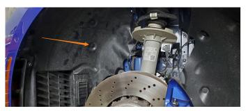
**3.** Using an 8mm socket, remove the two (2) bolts on each side of the vehicle that secure the bumper. Then, remove the two (2) plugs on the driver's side and the three (3) plugs on the passenger's side.
