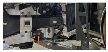
Lug studs: 140 N-m (103 lb-ft) torqued in a star pattern
