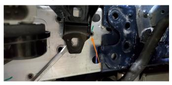
17. Place a drain pan under the transmission cooler lines to collect the transmission fluid when the lines are disconnected. Disconnect the two [2] lines from the transmission cooler by using an automotive pick to pull straight up on the green clips to unlock the fittings. The fittings can then be pushed off of the cooler. Then, using a T30 Torx socket, remove the two [2] bolts securing the cooler and remove it from the vehicle. Be sure to properly dispose of all used transmission fluid.
