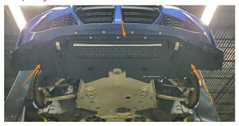
**5.** Using a 10mm socket, remove the bolts securing the engine skid plate and remove it from the vehicle.
