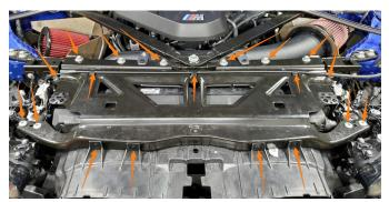
10. Using a 10mm socket, remove the bolt securing the air duct to the upper auxiliary radiator bracket on the driver's side of the vehicle. Then, using a 13mm socket, remove the two (2) bolts securing the upper auxiliary radiator bracket and remove the bracket from the auxiliary radiator. Then, remove the auxiliary radiator from the lower bracket and move it to the side. The auxiliary radiator can be secured to the vehicle with zip ties to prevent it from falling.
