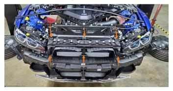
9. Remove the four (4) pop clips securing the shroud to the metal bracket. Then, remove the hood release cable from the clips in the bracket. Next, using 13mm, T30 Torx, & T40 Torx sockets, remove the twelve (12) bolts securing the metal bracket and remove it from the vehicle.
