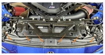
**7.** Using a T30 Torx socket, remove the eight (8) bolts securing the bumper to the vehicle. Then, remove the front bumper from the vehicle.
