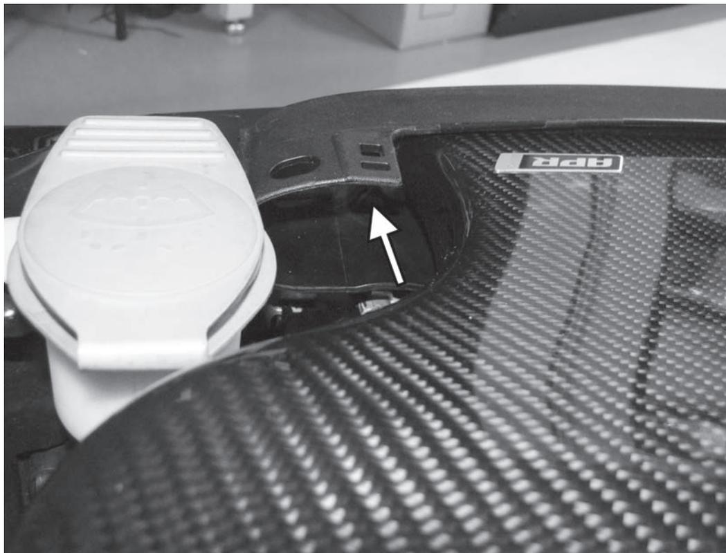
3) Remove the screw that holds the left side of the intake to the back of the radiator core support. Slide the intake out of the tab on the right hand side. Separate the intake from the back of the core support.
