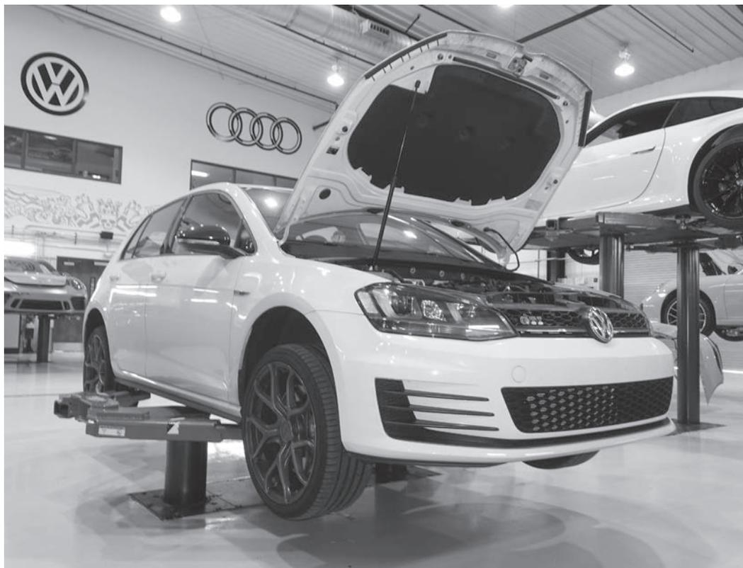
1) Securely place the vehicle on a lift or jack stands. Be aware that this install may require performing a wastegate adjustment using a factory scan tool or other device, such as VAG-Com.
