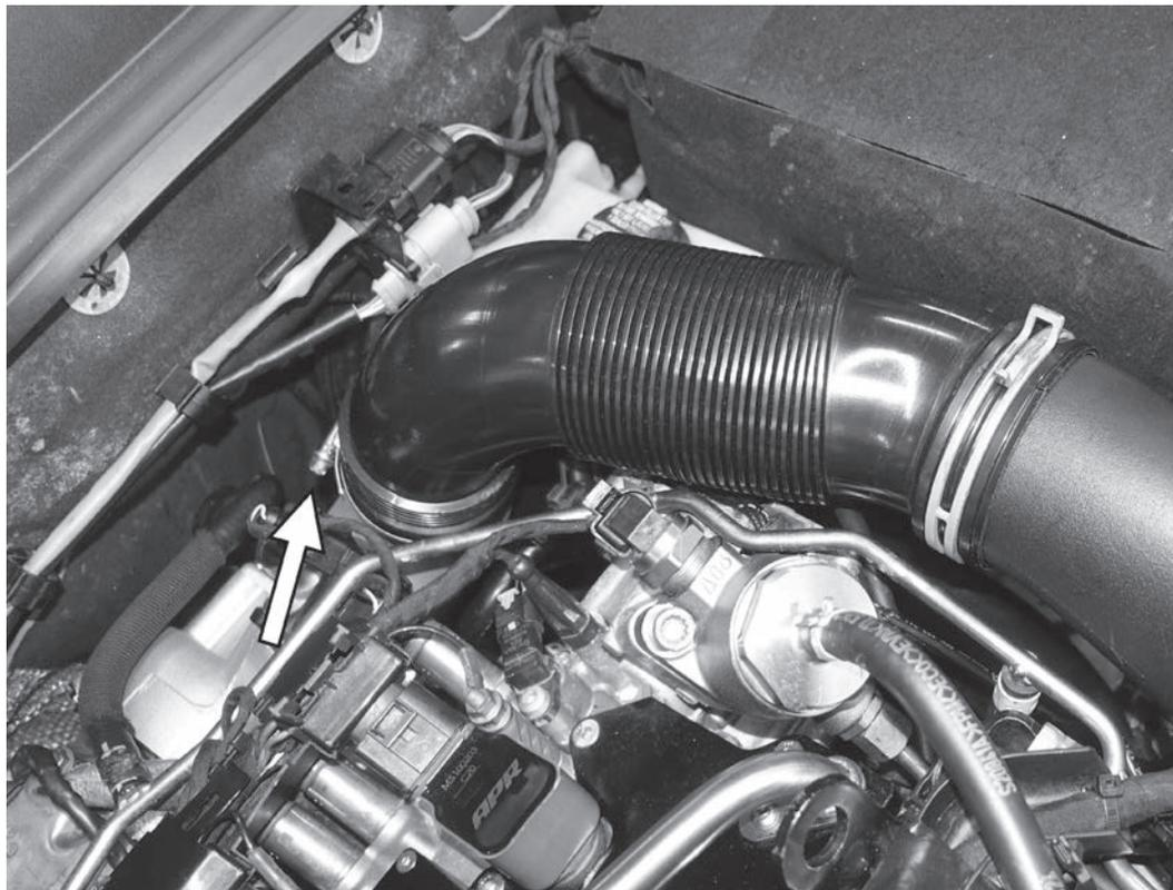
57) Reinstall the intake on the car. Tighten the 7mm screw on the clamp that connects the accordion inlet to the turbocharger. Reconnect the PCV hose to the turbo, or if equipped, the hoses to the APR catch can.
